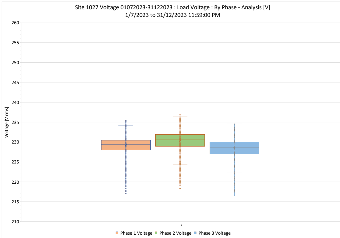
Figure 6 Average Grid Voltage - Box Whisker Plot – 3 phases - 1 minute average – 6 month period
