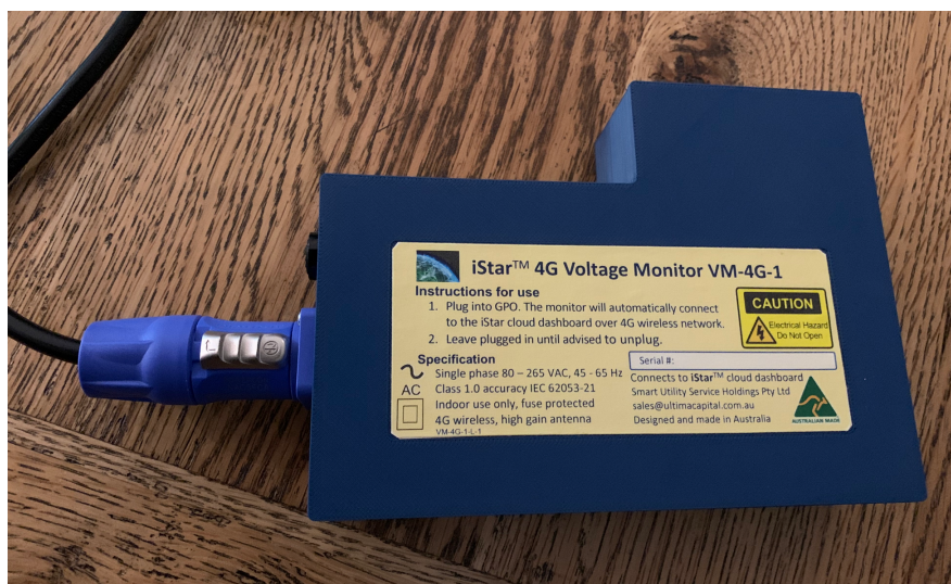
4G Voltage Monitor Case, showing latching input connector
