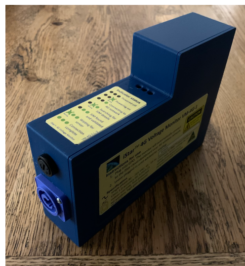
4G Voltage Monitor Case, showing latching input connector
